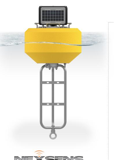
The **CB-75** Data Buoy is a compact, affordable, and easy to deploy platform for both water and atmospheric observations. At 21" (53.34cm) hull diameter and 40 lb. (18.14kg) weight, it's ideally suited for tethered moorings. The buoy is designed to integrate the **X3-SUB** Submersible Data Logger, which includes external sensor ports to support weather stations, thermistor strings, multi-parameter sondes, Doppler current profilers, GPS, and other monitoring instruments.
