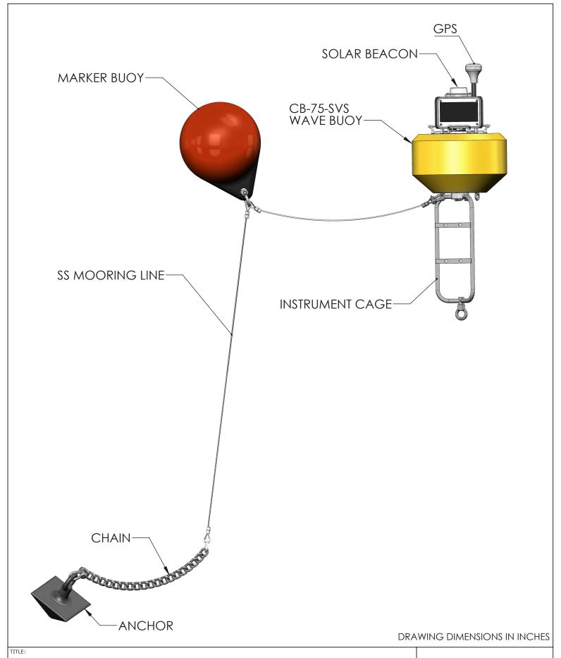
NEXSENS CB-75-SVS WAVE BUOY - TYPICAL WAVE MONITORING SYSTEM
