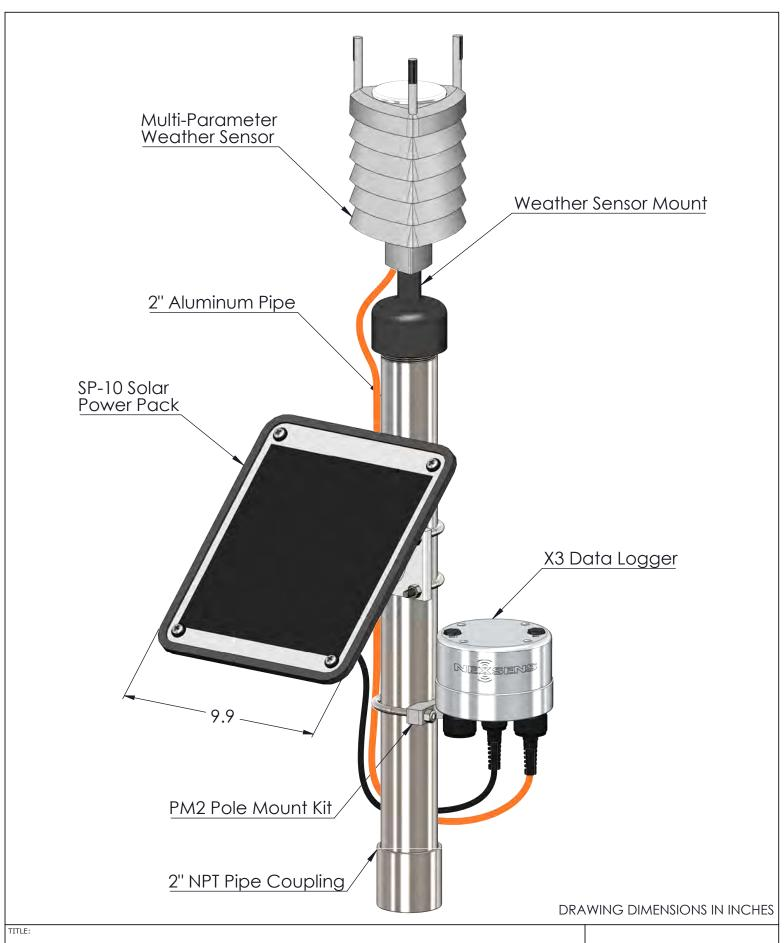
NEXSENS X3 DATA LOGGER - TYPICAL WEATHER SYSTEM
