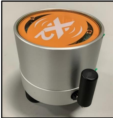
Figure 4: Iridium antenna connected to X2 antenna port.
