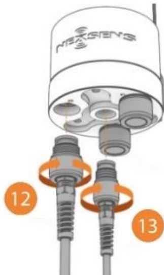
Figure 5: X2 Sensor (step 12) and power (step 13) connection.
