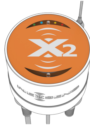
Figure 4: X2 LED light indicators.
