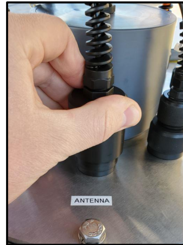
Figure 4 & 5: Iridium RF cable antenna connected to X2 antenna port.
