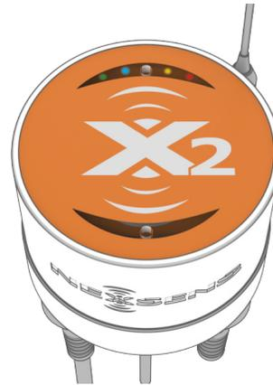
**Figure 3:** X2 LED light indicators located above the X2 logo on the clear top lid.
