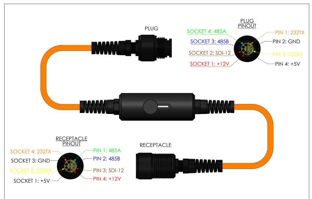
NEXSENS TS210 - SOCKET PINOUT
