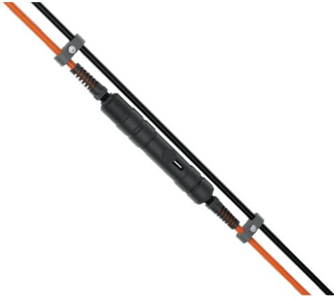
Figure 1: NexSens T-Node FR Thermistor String.
