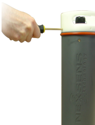
Figure 2: Remove the battery lid.
