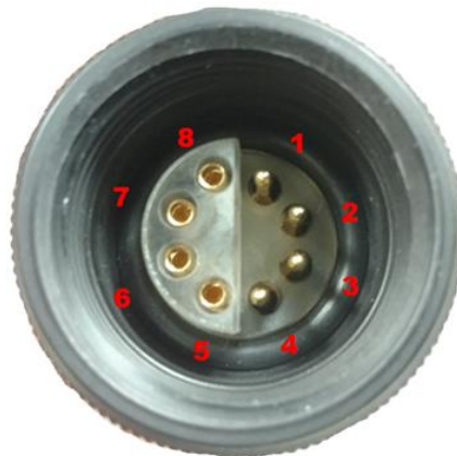
RAIN-RS485 Adapter Receptacle Pinout
