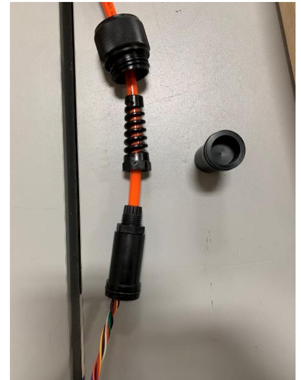
Sensor cable with UW-Bulkhead, PG-9 Flex Fitting, and corresponding UW Retainer (Removed UW Retainer to the right)
