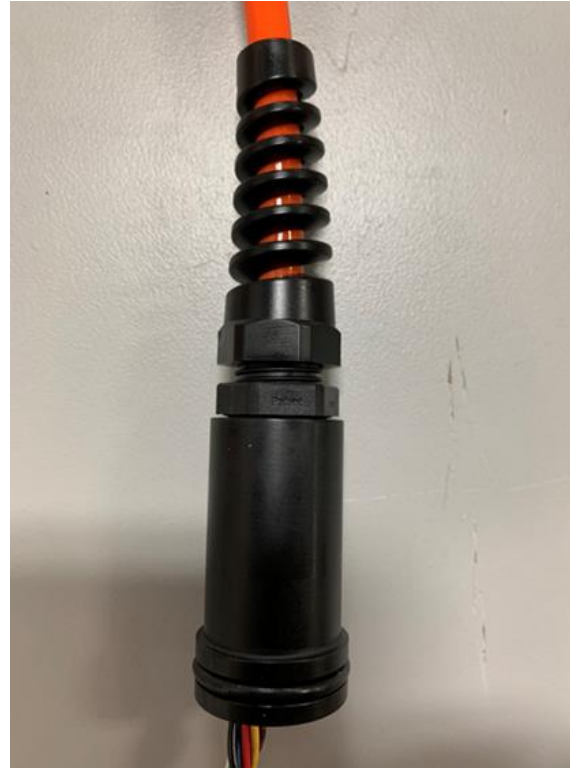
PG-9 Flex Fitting hand tightened on UW-Retainer
