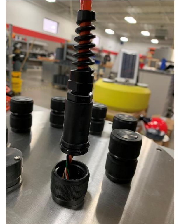
Routing wires through empty UW-Bulkhead port
