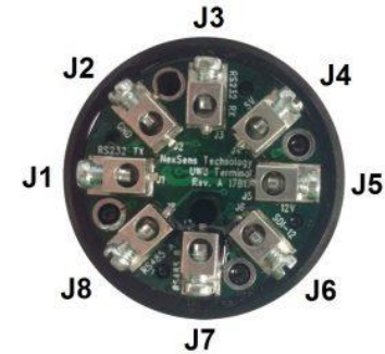
UW-FWP Terminal Pin Numbering
