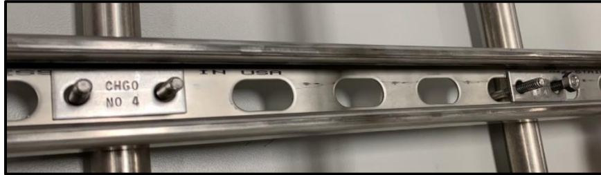
Figure 11: Top view of U-bolt and brace alignment on instrument cage.
