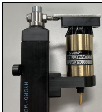
Figure 7: Side view of the Hydro-wiper with LI-COR 192 sensor inserted and sensor holder reattached.
