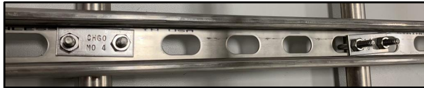
Figure 12: Complete Unistrut arm attachment to a small NexSens instrument cage.
