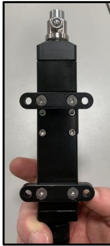
Figure 4: Back view of hydro-wiper; remove the 4 small bolts in the middle.
