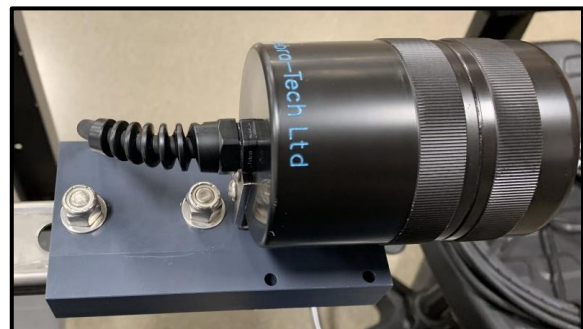
Figure 3: Top view of mounting block connected to the end of the Unistrut arm.
