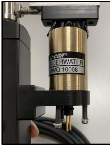
Figure 8: Side view of sensor holder with "shrink tube" screws partially inserted.
