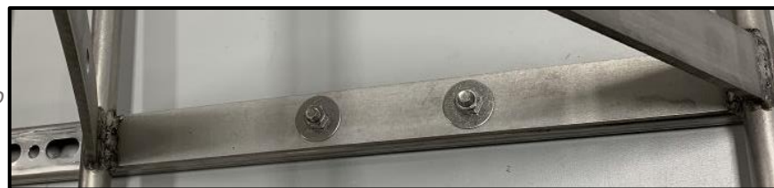
Figure 14: Complete Unistrut arm attachment to a large NexSens instrument cage.
