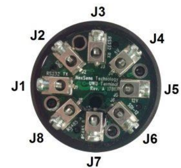
UW-FWP Terminal Pin Numbering
