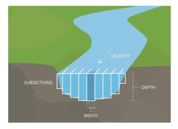
In addition to stage, discharge must also be established before streamflow information can be computed. Discharge is the volume of water moving down a waterway per unit of time. It is most commonly expressed in cubic feet per seconds or gallons per day. To calculate discharge, multiply the area of water in a channel cross section by the average velocity of water in that cross section. In short: discharge = area X velocity
