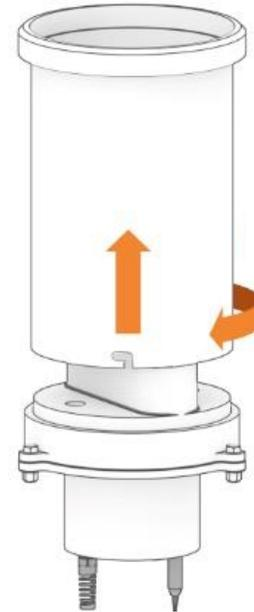
Rotate and lift the bucket gently during removal
