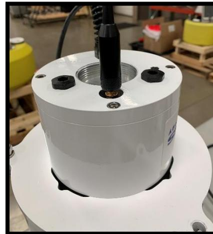
Connect the SMA antenna on the G2-RTU
