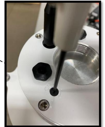
Twist the power plug to apply power with the battery pack
