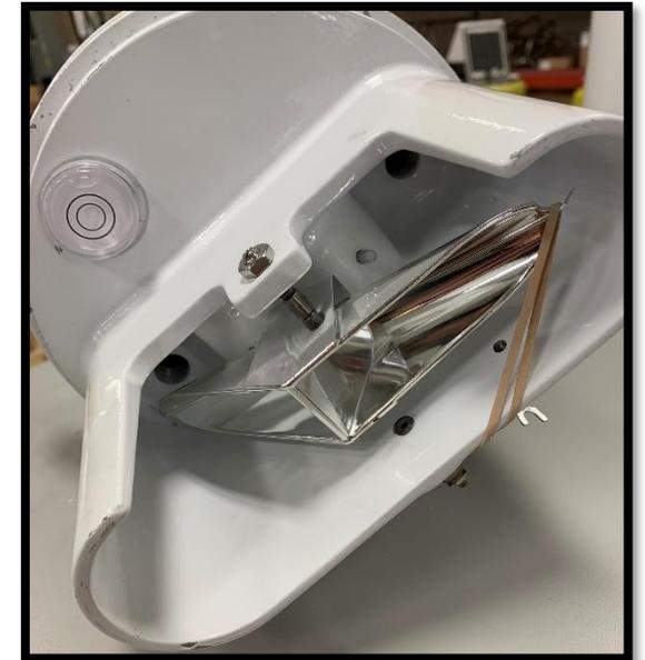
Remove the rubber band from the tipping apparatus
