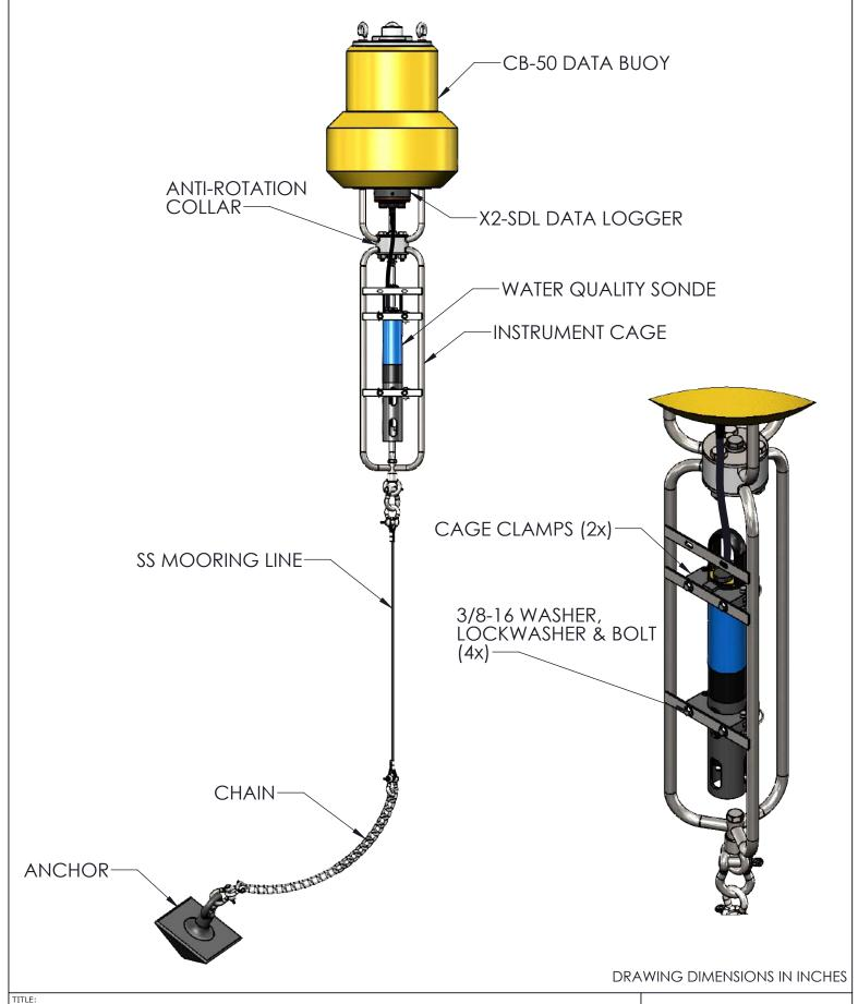
NEXSENS CB-50 DATA BUOY - TYPICAL WATER QUALITY MONITORING SYSTEM
