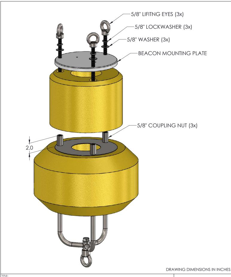
NEXSENS CB-50 DATA BUOY LID INSTALLATION
