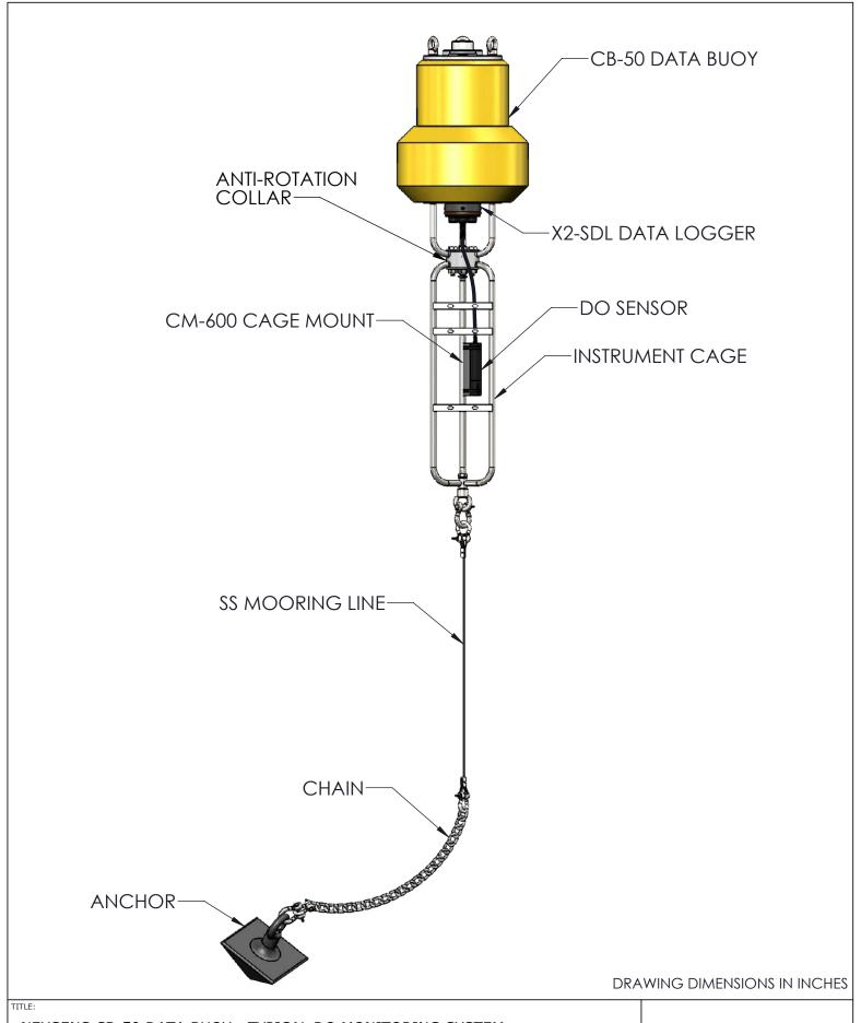
NEXSENS CB-50 DATA BUOY - TYPICAL DO MONITORING SYSTEM
