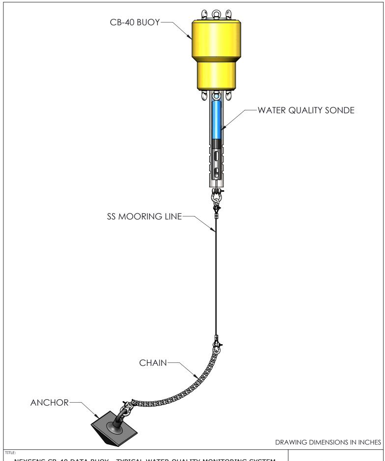
NEXSENS CB-40 DATA BUOY - TYPICAL WATER QUALITY MONITORING SYSTEM
