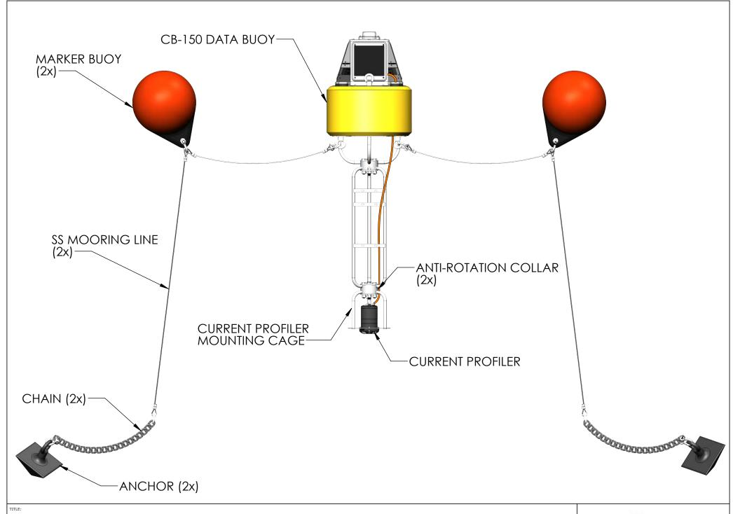
NEXSENS CB-150 DATA BUOY - TYPICAL CURRENT PROFILING SYSTEM
