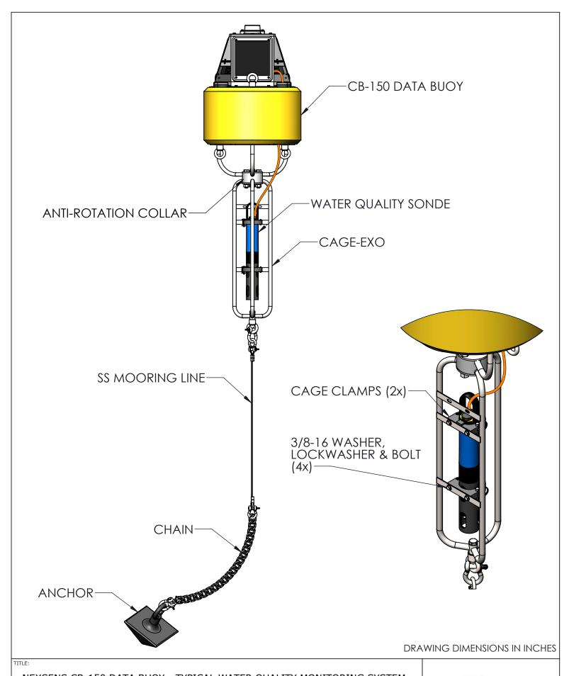
NEXSENS CB-150 DATA BUOY - TYPICAL WATER QUALITY MONITORING SYSTEM
