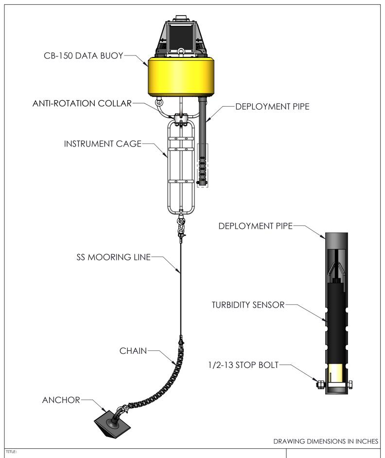
NEXSENS CB-150 DATA BUOY - TYPICAL TURBIDITY MONITORING SYSTEM
