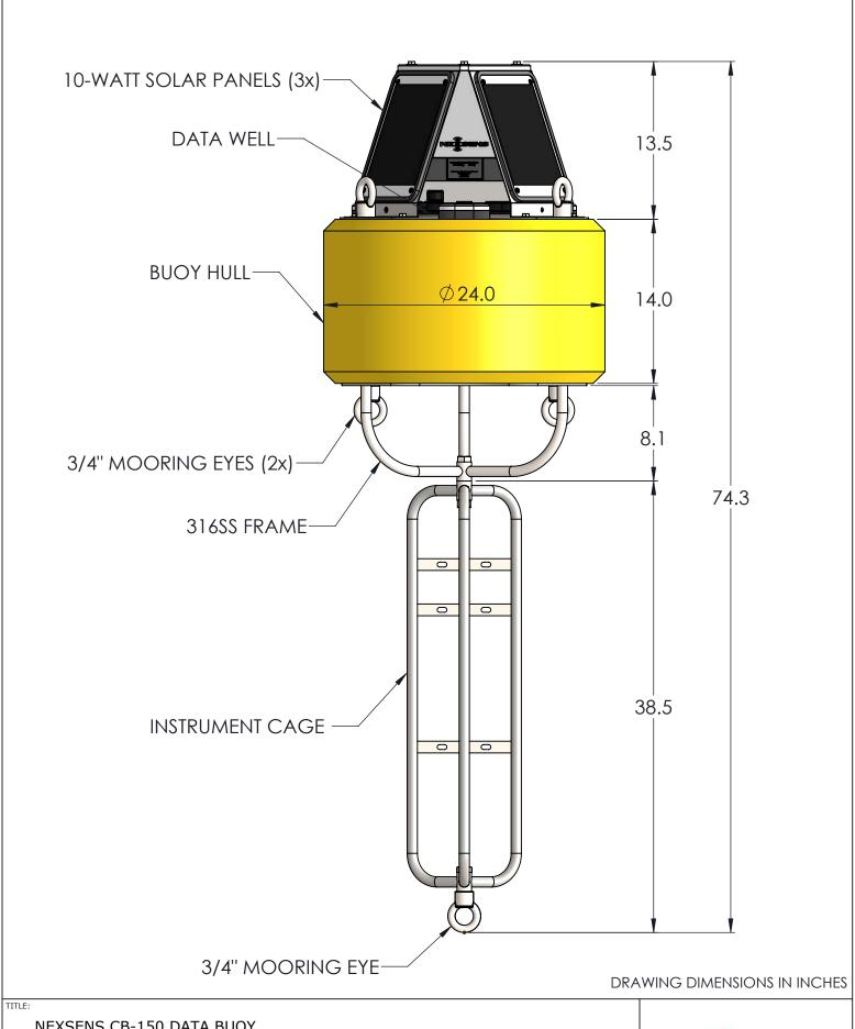
**NEXSENS CB-150 DATA BUOY**
