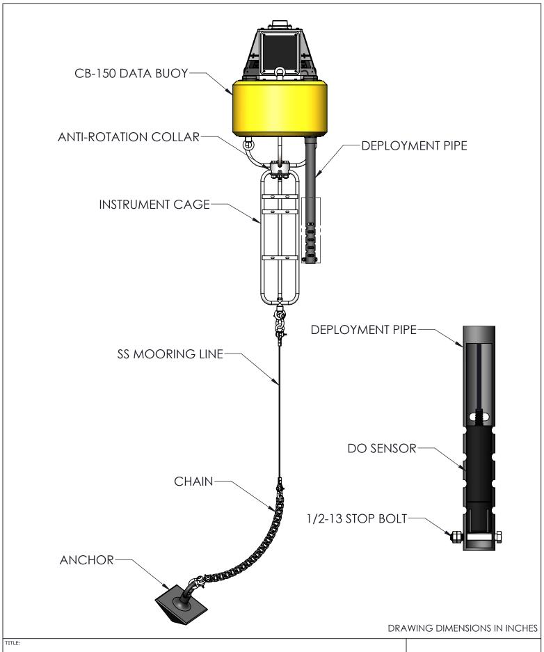
NEXSENS CB-150 DATA BUOY - TYPICAL DO MONITORING SYSTEM
