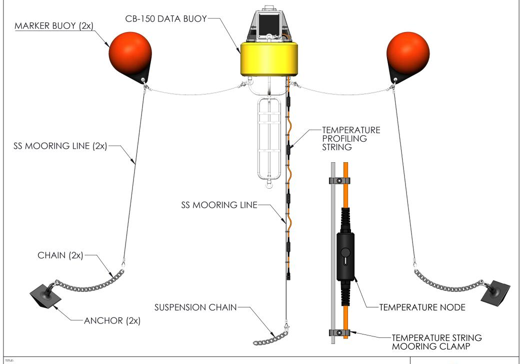
NEXSENS CB-150 DATA BUOY - TYPICAL TEMPERATURE PROFILING SYSTEM
