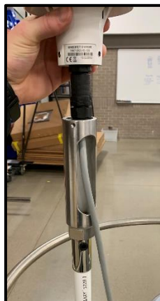
Figure 3: Routed GMX cable through the opening on the pole mount.
