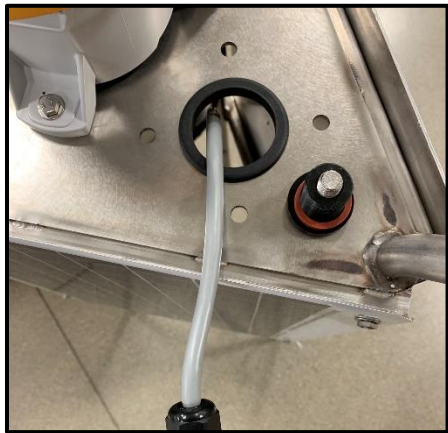
Figure 1: Top view of solar tower with routed GMX cable and pre-installed PVC base.
