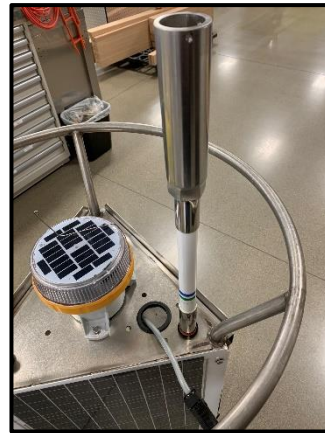
Figure 2: Top view of solar tower with attached CB-MXM-M.
