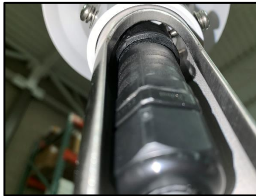
Figure 2: Internal view of the contact between the screws and the plastic Maximet connector. Screws should gently make contact with the connector.
