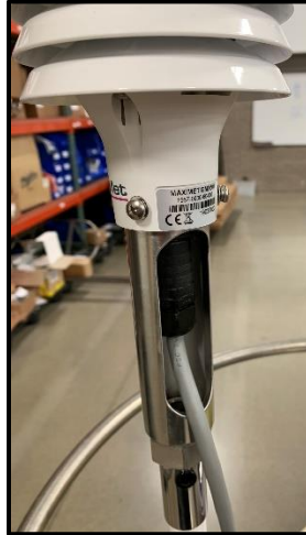
Figure 1: MaxiMet sensor mounted on the CB-MXM-M with screws inserted.
