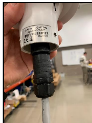
Figure 4: Closer view of the connector on the GMX cable.
