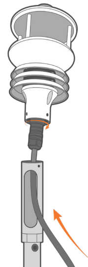
Figure 3: Connect the MaxiMet sensor cable.
