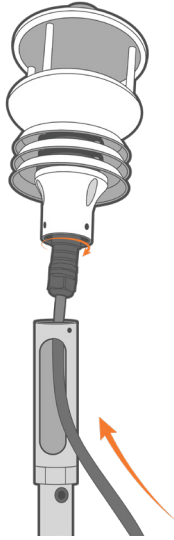
Figure 4: Connect the MaxiMet sensor cable.
