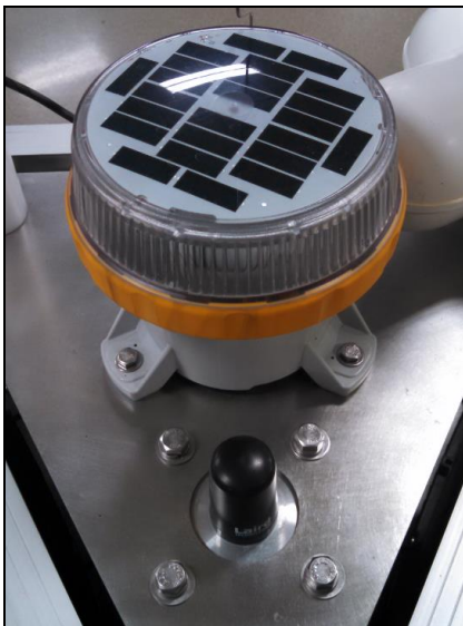
Figure 4: Tower with Beacon and RTU-C Module
