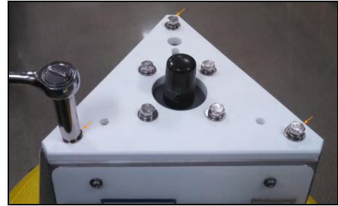
Figure 6: Top Plate Removal
