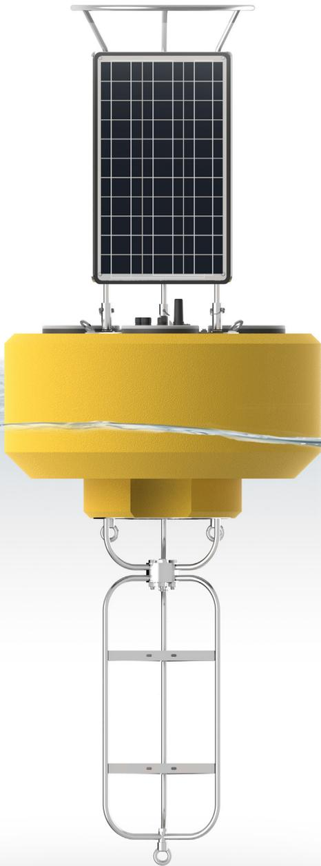
The NexSens **CB-1250** Data Buoy is designed for deployment in lakes, rivers, coastal waters, harbors, estuaries and other freshwater or marine environments. The floating platform supports both topside and subsurface environmental monitoring sensors including weather stations, wave sensors, thermistor strings, multi-parameter sondes, Doppler current profilers and other monitoring instruments.
