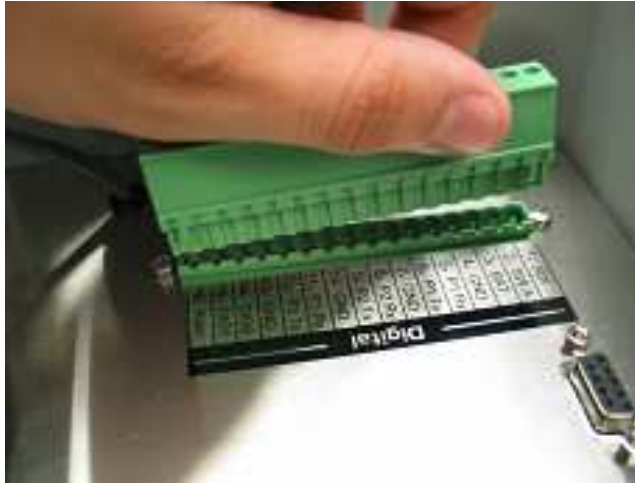
Figure 5: Unplug the green terminal strip from the data logger before wiring the sensor
