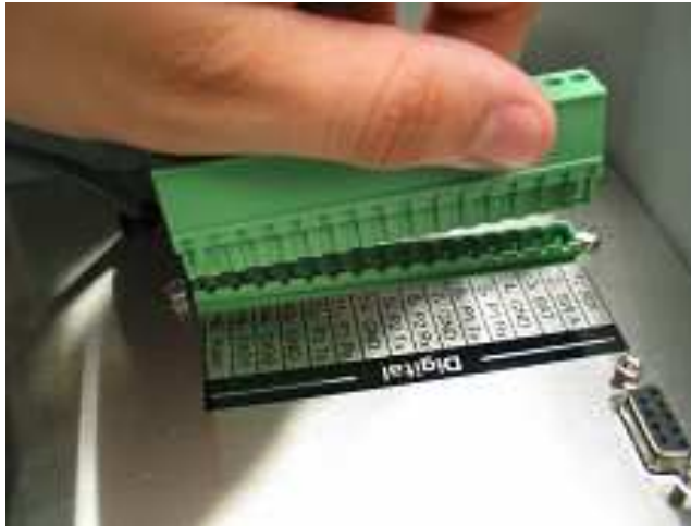
Figure 4: Unplug the green terminal strip from the data logger before wiring the sensor
