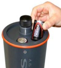
Figure 1: Installing batteries in the SDL500
