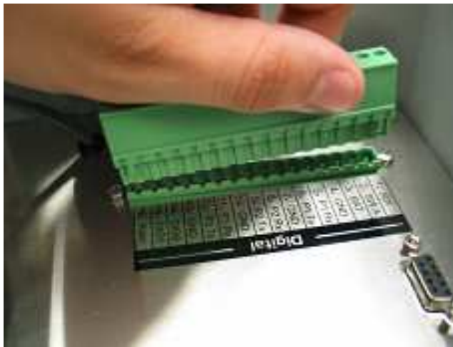
Figure 2: Unplug the green terminal strip from the data logger before wiring the sensor
