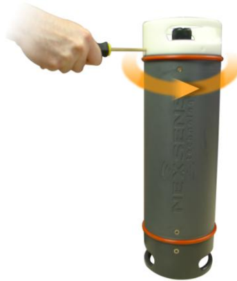
Figure 3: Unthreading the SDL500C battery lid from the communication bulkhead for battery installation
