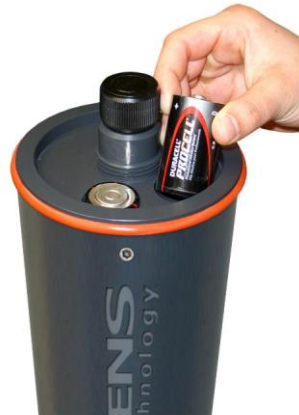
Figure 4: Installing batteries in the SDL500C
