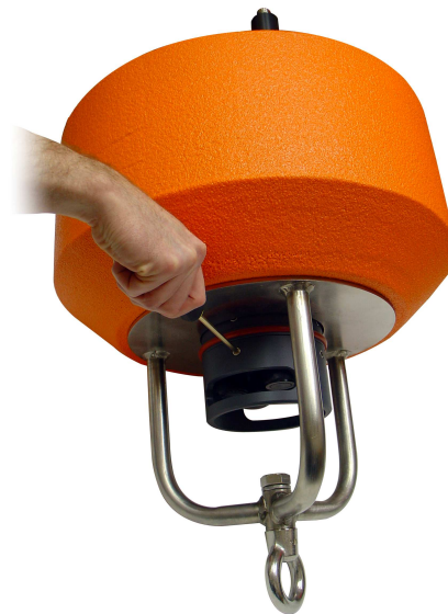
Figure 6: Removing bottom guard from SDL500 data logger using wrench from SDL maintenance kit
