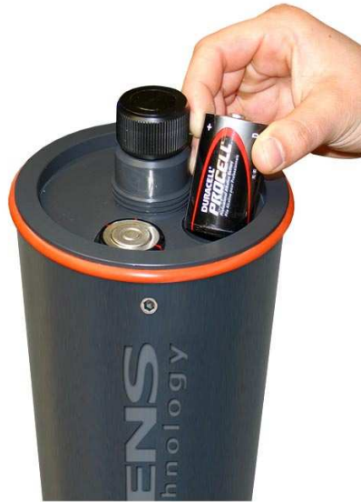
Figure 3: Installing batteries in the SDL500
