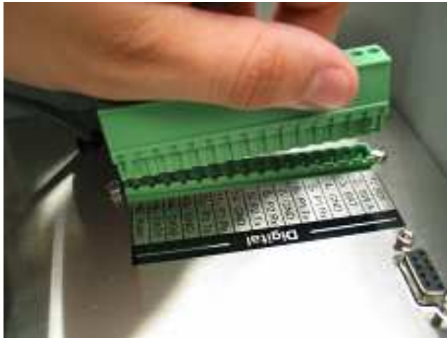
Figure 2: Unplug the green terminal strip from the data logger before wiring the sensor
