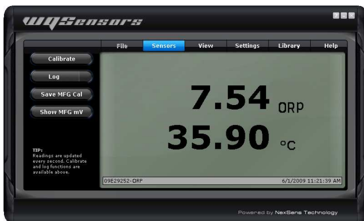
Figure 1: Click the Sensors tab to view live data; the connected sensor's serial number and time of last logged reading are displayed at the bottom of the screen
