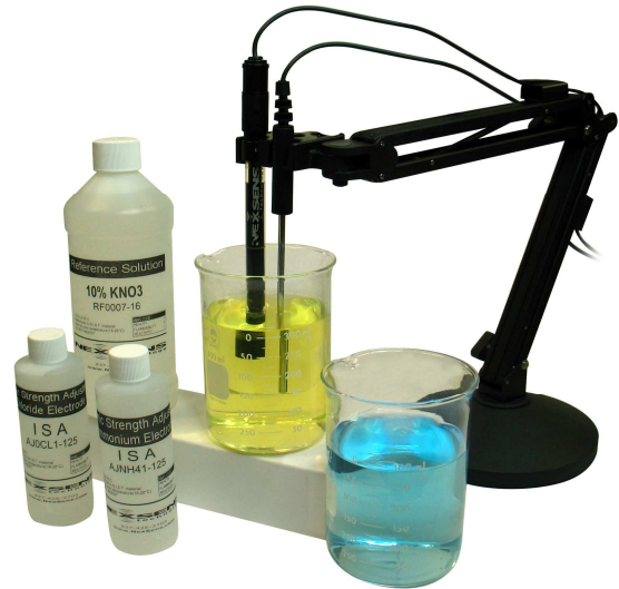
Figure 1: WQSensors secured in a WQ-A sensor arm
