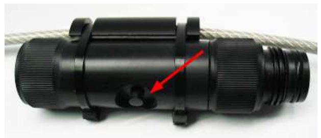
Figure 3: Securing the sensor using cable ties with temperature sensing tip pointed outward
