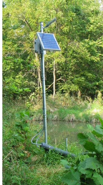
Figure 1: 902C locking well cap with top cable exit at slot
