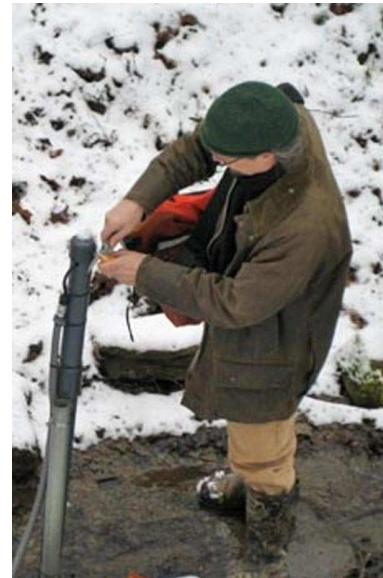
Figure 2: 904C locking well cap with top conduit connection
